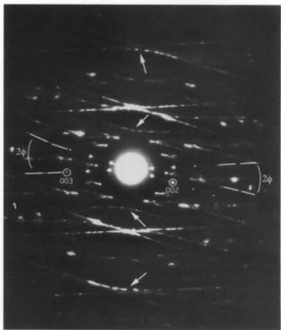
Fig. 25. Diffraction pattern of synthetic conically wound chrysolite fibre. Outward oriented V-shaped streaks are attached to all diffraction spots (except for the sharp 00l spots). The cone angle is 2\phi_0 \approx 19-20^\circ . Note the presence of hyperbola-shaped streaks as indicated by arrows.
